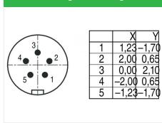
Contact arrangement (Plug-in side)
